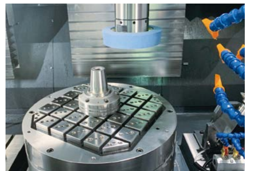
夾治具零件研磨 Fixture workpiece grinding
