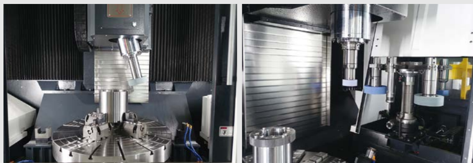
單主軸+擺頭機構 Single spindle + B axis
