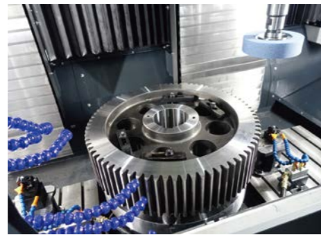
齒輪內外徑端面研磨 Gear ID, OD and flat grinding
