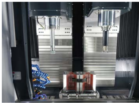
搪孔+內孔研磨 Boring + ID grinding
