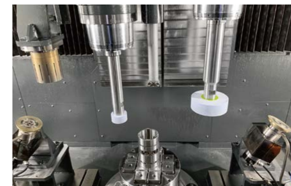
先車再磨 Turning + Grinding
