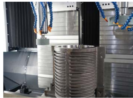
主軸箱內徑研磨 Spindle Housing grinding
