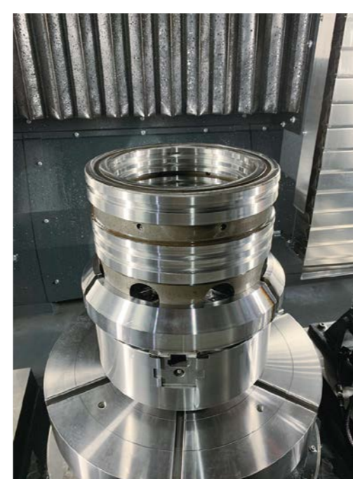
缸體研磨 Hydraulic cylinder grinding
