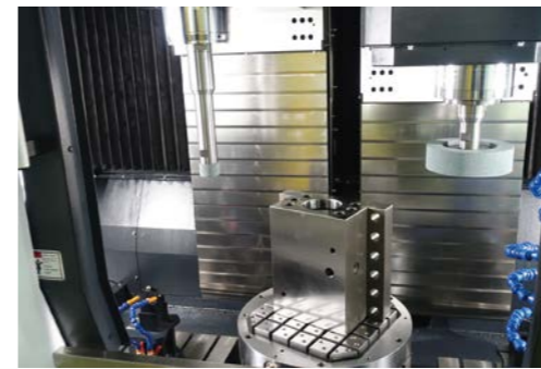
方形工件研磨內孔 Square workpiece grinding
