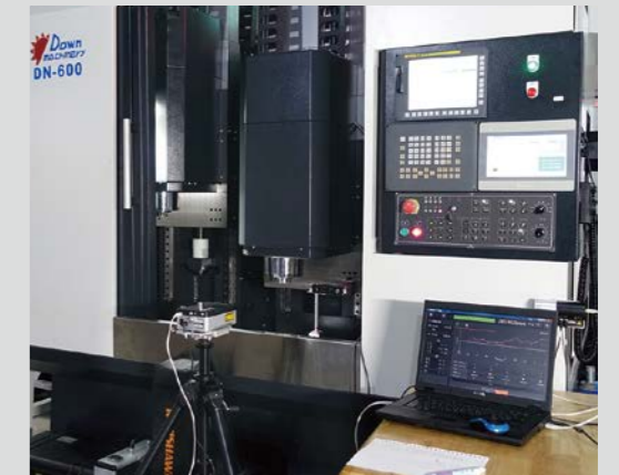
定位精度雷射檢驗 Position error measurement
