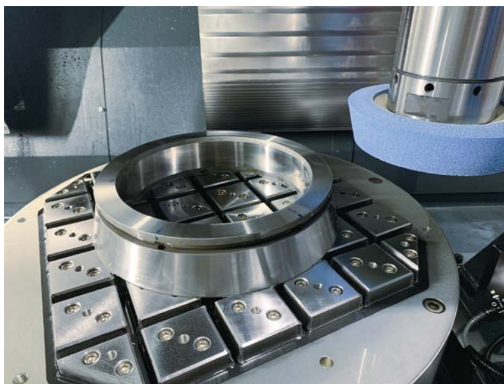
錐度及圓周上平面(逃邊)研磨 Taper and flat grinding
