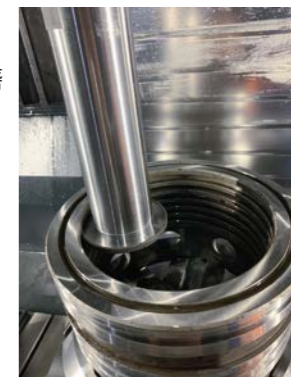
溝槽研磨 Groove grinding
