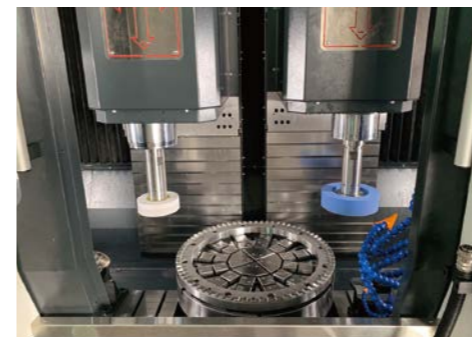
端齒圈內外徑研磨 End gear ring ID and OD grinding
