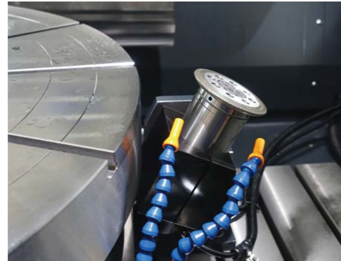
動力修砂 Power dressing
