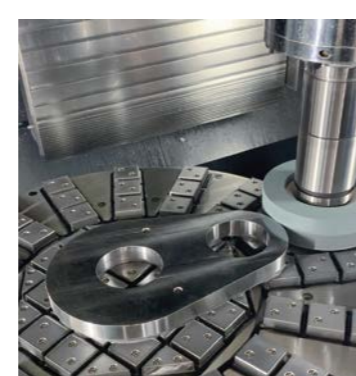
凸輪輪廓研磨(異形研磨) Cam profile grinding
